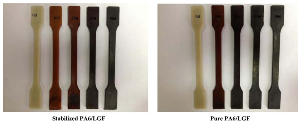
Figure 7. Digital photos of the PA6/LGF samples as a function of the aging time at 160°C. [Color figure can be viewed in the online issue, which is available at wileyonlinelibrary.com .]
